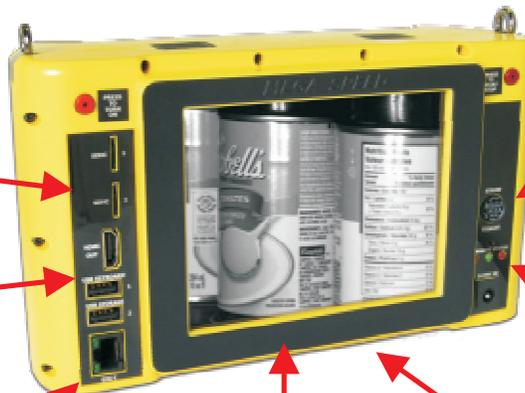
Sync in/ sync out, triggers, frame marker ADC & IRIG-B input options available
